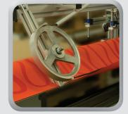
PVC spline from large rolls can be fed into the seam as it is sewn, with automatic cutting at end of seam.
