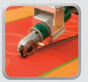
Built-in round knife cutter automates cutting of valance strip from the awning sheet.
